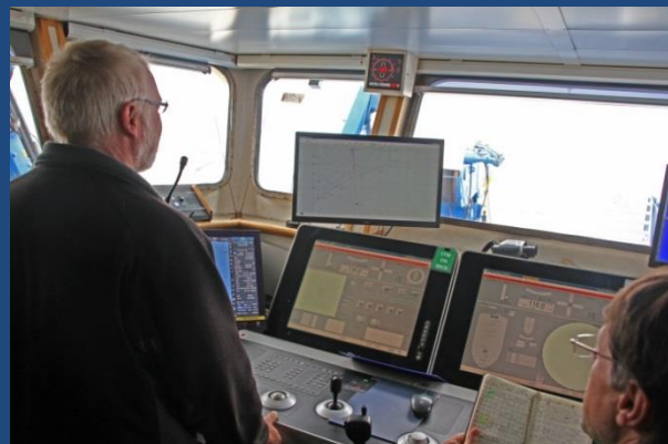
Each department on board the RS Sentinel is equipped with a client computer running QINSy to assist with their job tasks. Those clients are controlled by the host QINSy computer located in the survey office, to support ROV & Dive Control and the DP Bridge (as shown in the photograph).
