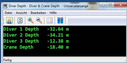
USBL beacons are mounted on diving equipment, the ROV and crane hook.
